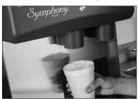
SensorSAFF not recommended for use with clear containers or for applications in direct sunlight
