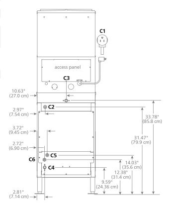
Measurements shown are with base stand legs at lowest position
