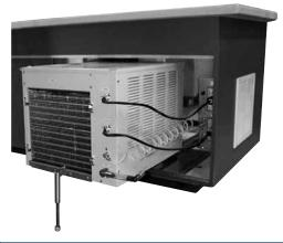
Slide-out accessory for Maestro ice machines with RIDE™ technology facilitates installation and service. Utility distribution panel allows easy connection of electric, incoming water and drain. Flexible connections from panel to ice machine allow ice machine to slide out for cleaning and service without disconnecting utilities. Includes front leg to support ice machine.
