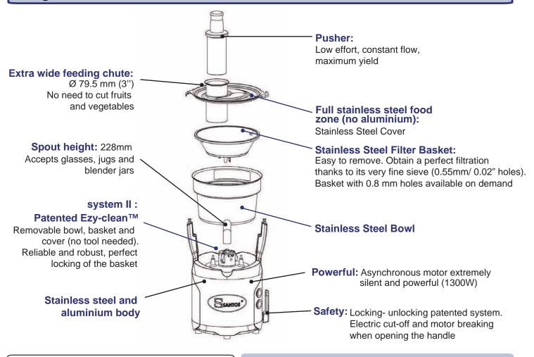
For all fruits and vegetables (citrus fruits must be peeled). Continuous juice production by centrifugal action and automatic pulp ejection.
