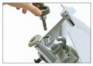
To degrease and dress the grinding stone simply pull it out.
