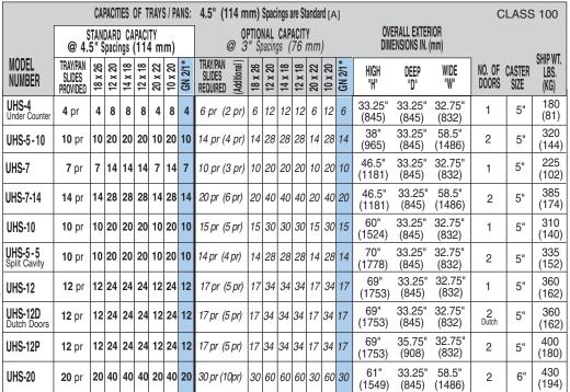
[A] Universal tray slides accommodate: (1) 18" x 26", (2) 12" x 20", (2) 14" x 18", (2) 12" x 18", (1) 20" x 22", (2) 10" x 20" trays/pans. Uprights punched on 1.5" (38 mm) centers. Universal tray slides are adjustable. Number of tray slides are listed above. Standard spacings are 4.5" (114 mm).
