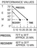
Precool Time is based on interior cabinet at 75°F. Values are for mid-size model listed.
