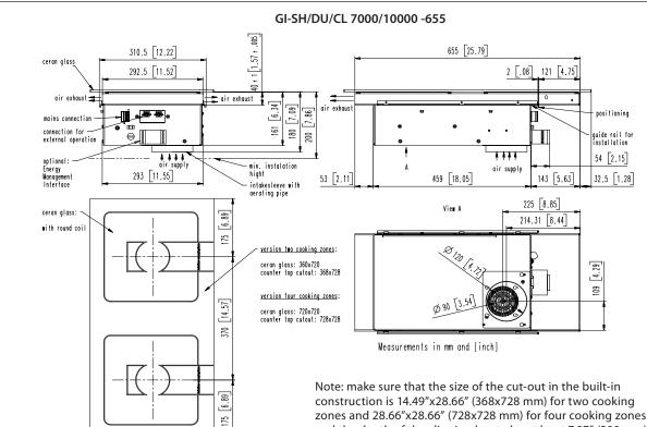
zones and 28.66"x28.66" (728x728 mm) for four cooking zones and the depth of the clipping has to be at least 7.87" (200 mm).
