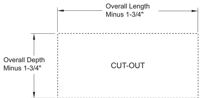
EXAMPLE: A DI-DP12X24 which measures 12" x 24" would require a cut-out size of 10-1/4" x 22-1/4"
