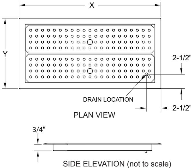
Make cut-out 1-3/4" smaller than the outer flange dimensions. This will leave approximately 1/8" gap between edge of cut-out and the drain pan sides for a snug fit.
