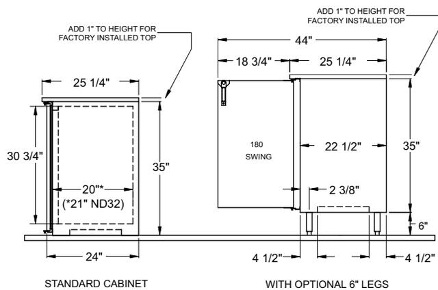
Note: Available with compressor left or right. Compressor left model shown. Use Model Number Key to specify location when ordering.
