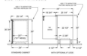
Note: Available with compressor left or right. Compressor left model shown. Use Model Number Key to specify location when ordering.
