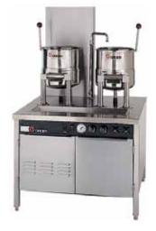
kettles. ASME Code constructed and National Board registered for operation up to 15 PSI. 200,000 BTU boiler delivers to 120,000 BTU/hr into the product, is 60% efficient and delivers 3.7 boiler horsepower. Unit comes with standing pilot. Electronic ignition is available as an option. Auxiliary manual drain valve to simplify maintenance is also included.
