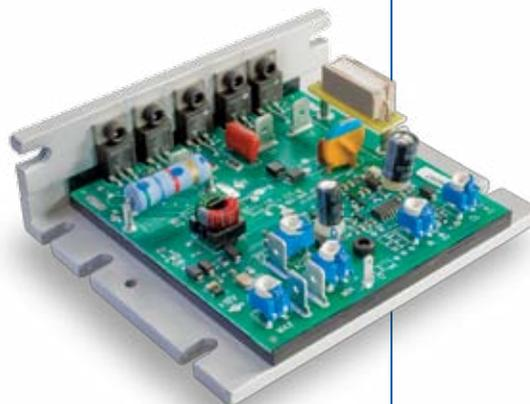
Special electronic control helps maintain constant speed regardless of load
