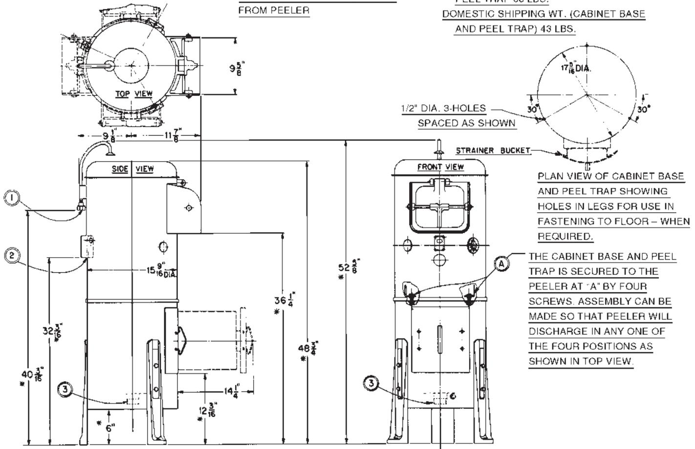
PLAN VIEW OF CABINET BASE AND PEEL TRAP SHOWING HOLES IN LEGS FOR USE IN FASTENING TO FLOOR – WHEN REQUIRED.
