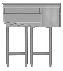
**DDU38***e* **Direct Drive Unloader.** Center pawl to be connected to dishwasher conveyor by means of a stainless steel adjustable rod. As conveyor drives, center pawl drives racks around 90 degree corner. The DDU38*e* is designed to move the racks at the same speed as the conveyor dishwasher speed. The DDU38*e* adds 38" to the length of the machine.
