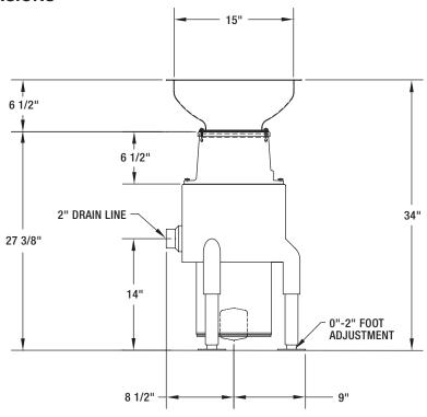
NOTE: Accessory Groups A and B – 18" Cone is Standard. Specify 15" Cone in Place of 18" Cone When Desired.
