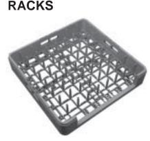
P-1400 Tray Rack. 20" x 20" pegtype with one open end. All plastic construction. Will handle trays up to 16" x 22" in standard height C-Line models. Will handle 18" x 26" bun pans in C-Line model 3" higher than standard. For 16" x 22" trays in AM series straight-through machine, or maximum of 16" x 20" in AM corner machine. Specify tray size when ordering. Will not handle oval trays.
