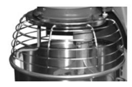
The scraper is used in conjunction with the B Beater or Wire Whips. While the agitator is mixing the product, the scraper is continuously scraping the inside of the mixer bowl. No more stopping mid-cycle to manually scrape down the sides of the bowl. The bowl scrapers are built to last and are made of urethane elastomer. The optional bowl scraper is available for the following models: HL120, HL200, D300, D340, HL600, HL800 and HL1400.
