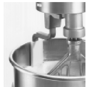
H600 with Scraper Option - Bowl in down position
