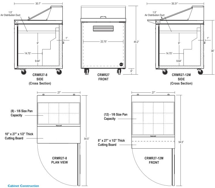
The exterior cabinet top, front, and sides, are constructed of high quality stainless steel.
