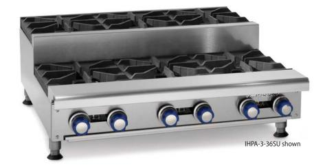
OPEN BURNERS - PyroCentric™ 32,000 BTU (9 KW) anti-clogging burner with a 7,000 BTU/hr. (2 KW) low simmer feature. Two rings of flame for even heating.
