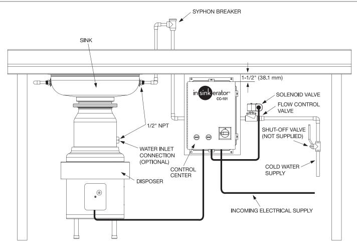
NOTE: The CC-101 control center should be mounted 1-1/2" (38.1 mm) back from the front surface of the table.
