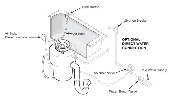
NOTE: InSinkErator Commercial Air Switch (Part No. 13754) is available for 120V model only.
