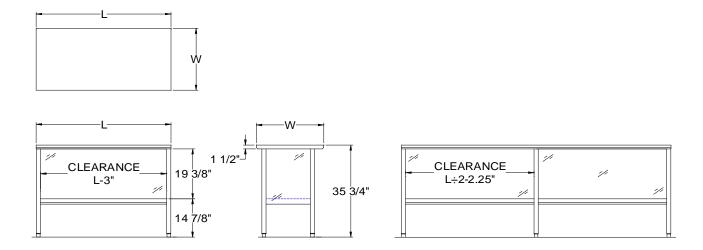
Shipped Welded Set-Up Units 7 ft. and larger are furnished with six legs. All dimensions are typical. Tolerance +/- .500". Finished size of undershelf. Shelf length = length minus 4.875" Shelf width = width minus 4.25"
