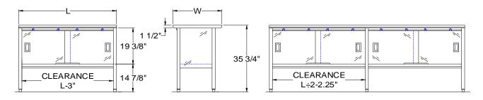
Shipped Welded Set-Up Units 7 ft. and larger are furnished with six legs. All dimensions are typical. Tolerance +/- .500". Finished size of undershelf. Shelf length = length minus 4.875" Shelf width = width minus 4.25"
