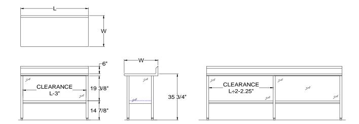
Shipped Welded Set-Up
