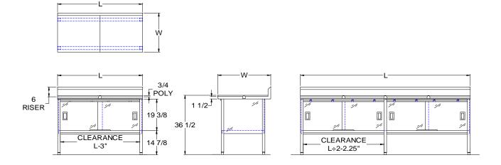
Shipped Welded Set-Up Units 7 ft. and larger are furnished with six legs. All dimensions are typical. Tolerance +/- .500".
