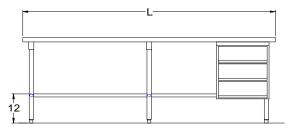
Shipped Knocked down Units 7 ft. and larger are furnished with six legs. All dimensions are typical. Tolerance +/- .500".
