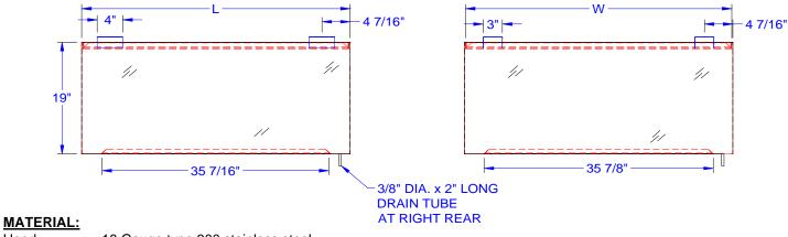
Hood: 18 Gauge type 300 stainless steel Baffle: 18 Gauge type 300 stainless steel
