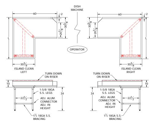
All units ship unassembled for reduced shipping cost. Units 7 ft. and larger are furnished with six legs.
