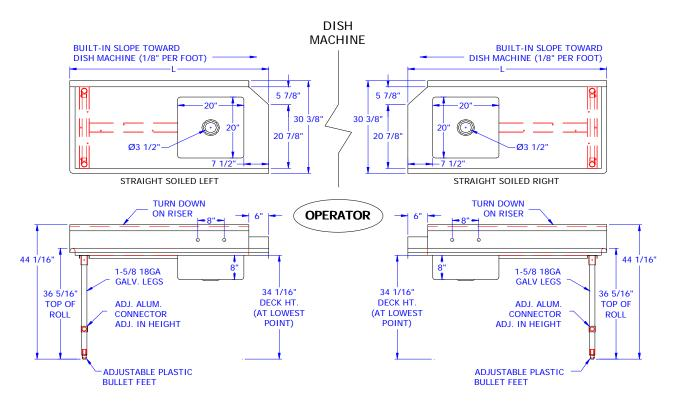
All units ship unassembled for reduced shipping cost. Units 7 ft. and larger are furnished with four legs. All dimensions are typical.
