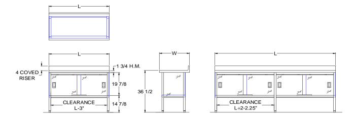
Shipped Welded Set-Up Units 7 ft. and larger are furnished with six legs. All dimensions are typical.
