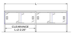
Shipped Welded Set-Up Units 7 ft. and larger are furnished with six legs. All dimensions are typical. Tolerance +/- .500". Finished size of undershelf. Shelf length = length minus 4.875" Shelf width = width minus 4.25"
