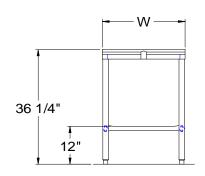
Shipped Standard Welded Set-Up Units 7 ft. and larger are furnished with six legs. All dimensions are typical.
