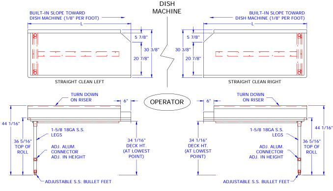
All units snip unassembled for reduced snipping cost. Units 7 ft. and larger are furnished with four legs. All dimensions are typical.
