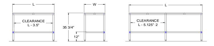
Shipped Standard Welded Set-Up Units 7 ft. and larger are furnished with six legs.
