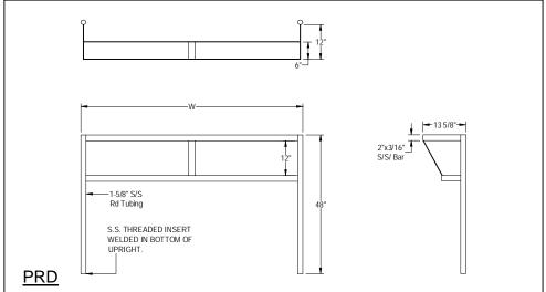
Shipped Welded set-Up
