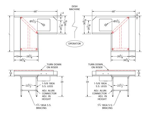
All units ship unassembled for reduced shipping cost. Units 7 ft. and larger are furnished with six legs.
