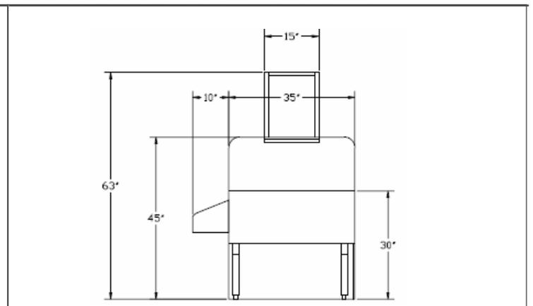
**MECHANICAL REQUIREMENTS:** 1/2" IPS Hot and Cold Water 1" IPS drain connection without Cold Plate. 1/2" IPS drain connection with Cold Plate. 1 1/2" IPS drain connection on Sink Bowls.
