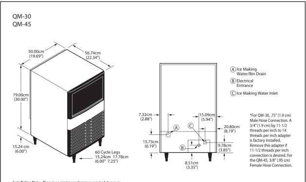
Installation Note - There is no minimum clearance required, however recommended clearance for top, sides, and back is 5" (12.7 cm).
