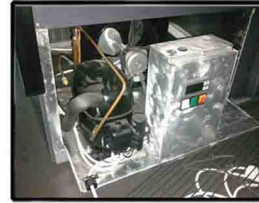
PULL OUT CONDENSING UNIT ON SELF CONTAINED
