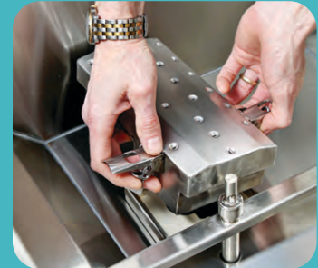
Stationary spray box simply unlatches for easy visual inspection and cleaning.
