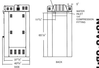
Allow four inches on each side and back of unit for
