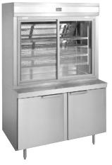
REFRIGERATION: Base and upper structure supplied with separate refrigeration coils. Expansion valve and refrigeration lines provided and installed for connection at PNL area (specify refrigerant if other than R-134a). Condensing unit not provided.
