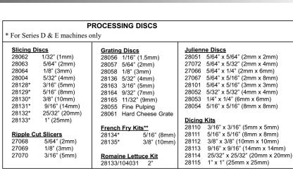
OPTIONAL EQUIPMENT: 36 additional processing discs and single or multiple disc rack or wall-mounted disc rack.
