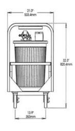
Minimum Wall Clearance Both Sides and Back -6 inches (152 mm)
