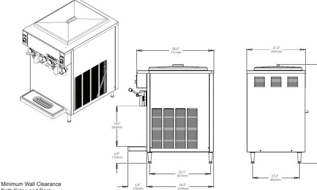
Minimum Wall Clearance Both Sides and Back -6 inches (152 mm)
