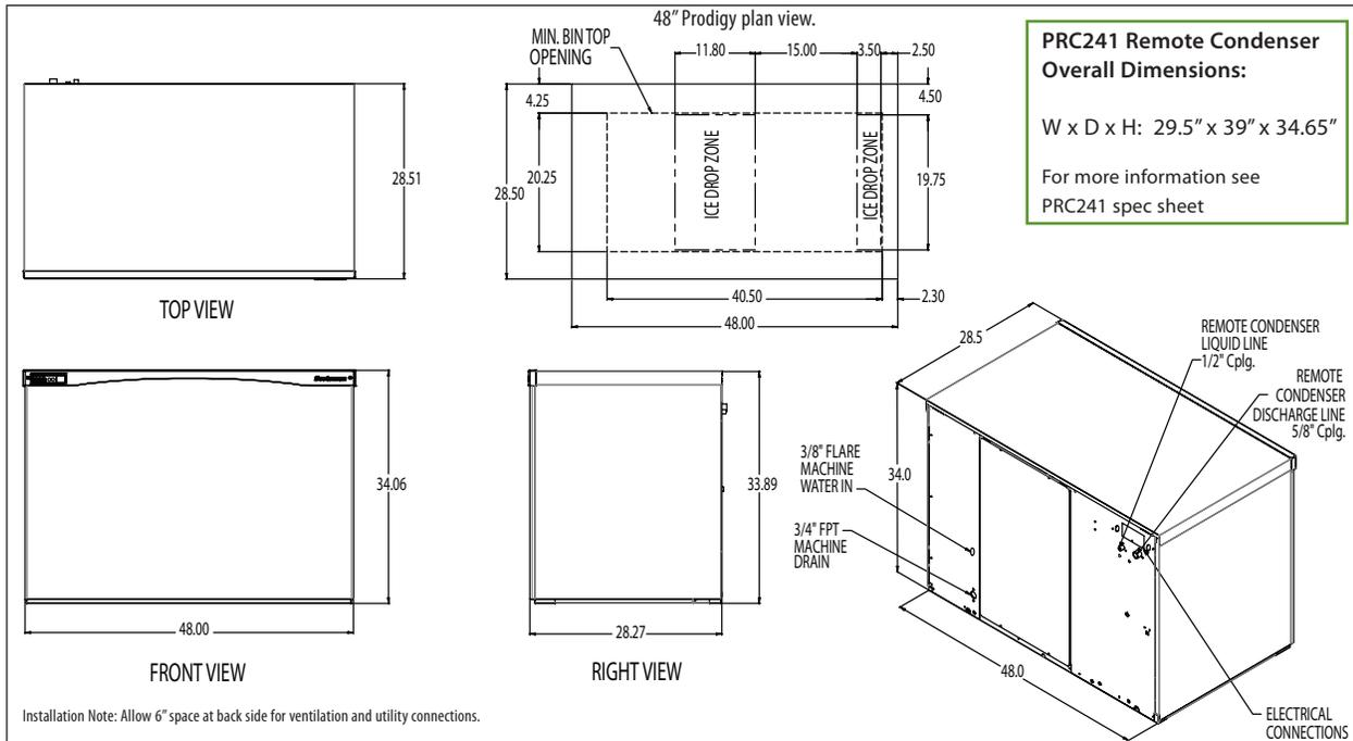
Installation Note: Allow 6" space at back side for ventilation and utility connections.
