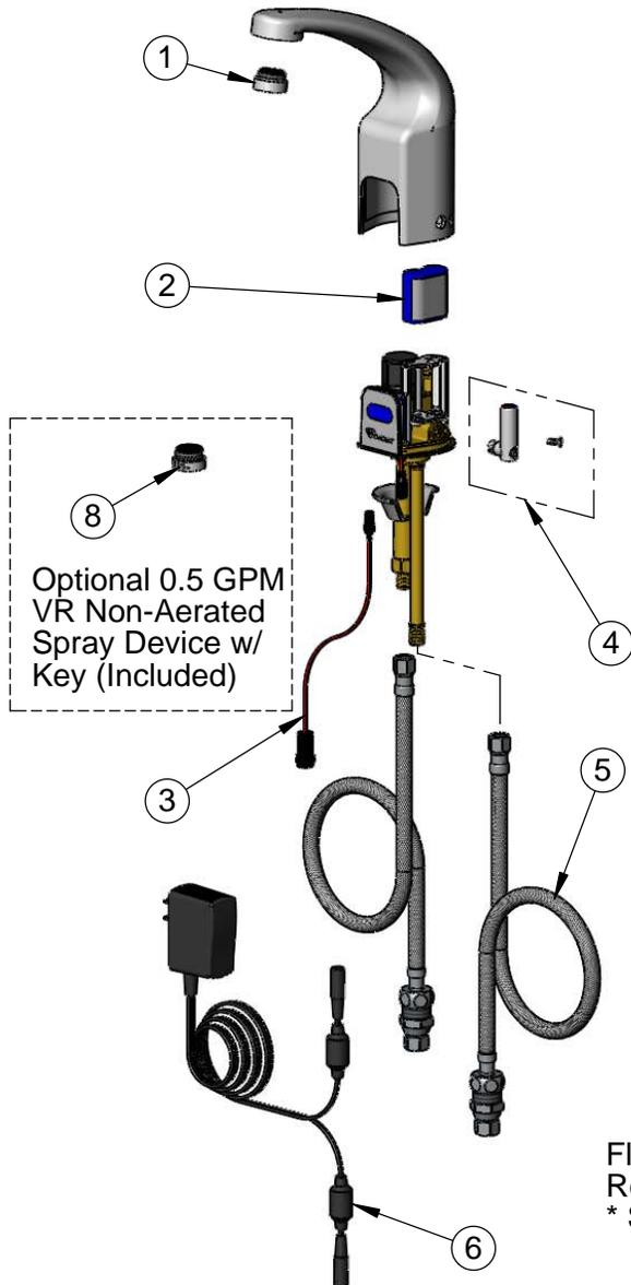
Optional 0.5 GPM VR Non-Aerated Spray Device w/ Key (Included)
