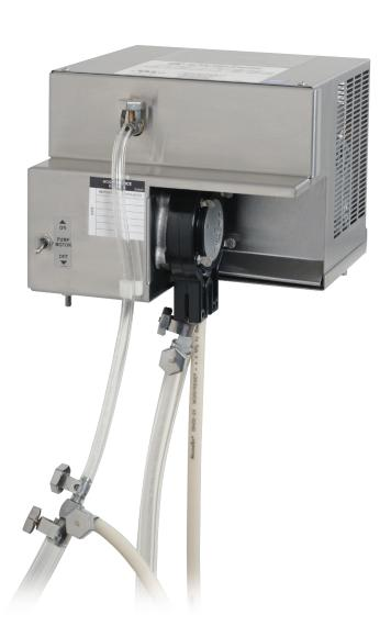
The U3 pump is the simplest pump available. No disassembly required for cleaning. The U3 pump has a capacity of 36 gallons per hour of standard soft serve or shake mix with an adjustable overrun. For use with all remote soft serve and shake freezers.
